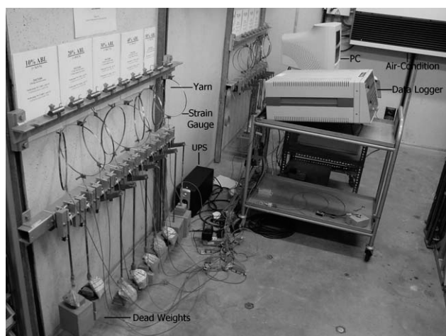
Figure 6 Experimental set-up for CCT tests.
